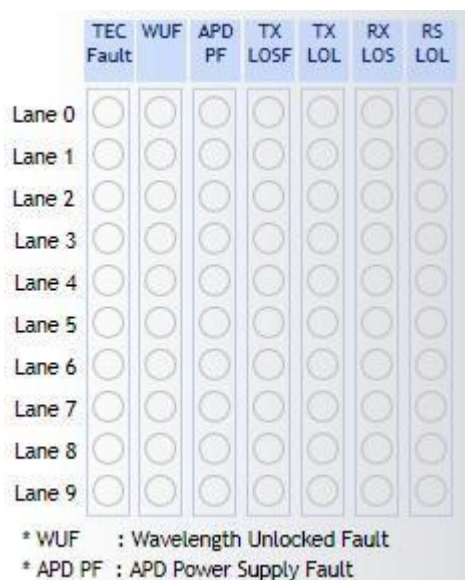
Figure 21 Network Lane n Fault and Status corresponding LEDs
